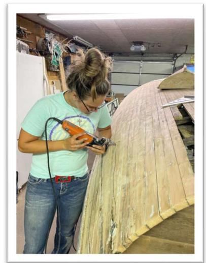
When I started to put the new boards in place, we ran into complications, like realizing that the boat was bent out of shape and none of the boards were the same size. The boat was very heavy as we had to flip it over multiple times to work on it. It was very deep from keel to deck making it hard to flip it in our garage.
