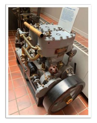
Photo: Engine from the front showing a large flywheel Credit: Paul von Goertz
